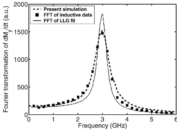
FIG. 3. Fourier transformation of the simulated time dependence of the inductive response in the CoFeHfO film superimposed on the experimental data from [17]. The simulation curve is normalized to match experimental data at low fields. Simulation parameters:  $D_z = 100$  nm,  $g = 2.15$ ,  $M_s = 800$  emu/cm<sup>3</sup>,  $H_{\text{appl}} = 40.2$  Oe,  $H_K = 56.5$  Oe,  $\alpha = 0$ ,  $\sigma = 100$  Å,  $R = 3$  μm.
