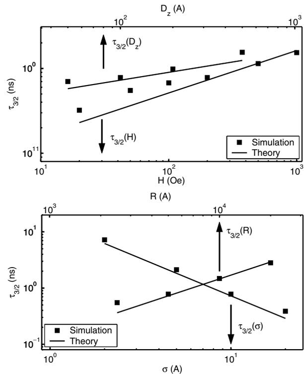
FIG. 2. The dependence of the decay time  $\tau_{3/2}$  on the applied field  $H_0$ , film thickness  $D_z$ , surface roughness standard deviation  $\sigma$ , and correlation length  $R$ . Calculation parameters same as in Fig. 1.
