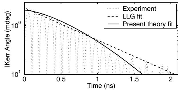
FIG. 4. LLG ( $\alpha_{\text{LLG}} \approx 0.0073$ ) and present theory ( $\tau_{3/2} \approx 0.77$  ns) fits to the experimental data. Fe<sub>0.5</sub>Co<sub>0.5</sub> film,  $D_z = 185$  Å,  $M_s = 1900$  emu/cm<sup>3</sup>,  $H_{\text{appl}} = 110$  Oe.
