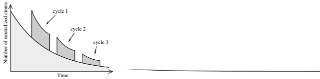
FIG. 3. A timing diagram of the experiment. The light grey area represents the collisional detachment contribution. The dark grey areas show the contribution due to the photodetachment of the excited state for three separate ring cycles.
