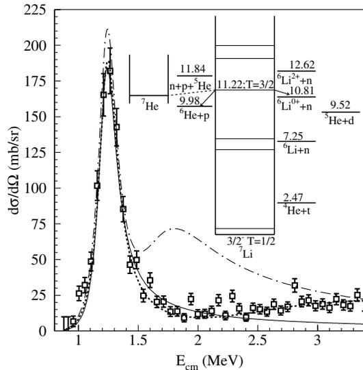
FIG. 3. The excitation function for the  ${}^6\text{He}(p, n){}^6\text{Li}(0^+; T = 1)$  reaction measured at  $180 \pm 8^\circ$ . See the text for a discussion of the curves. The inset shows the decay channels for the  $T = 3/2$  resonances in  ${}^7\text{Li}$ .
