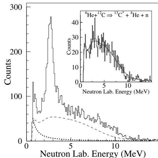
FIG. 2. The spectrum of neutrons in coincidence with  ${}^6\text{He}$  and a  $3.56 \pm 0.30\text{ MeV}$   $\gamma$  ray, measured with a  $(\text{CH}_2)_n$  target. The inset shows a neutron spectrum obtained with a natural carbon target. The contribution of the carbon background is shown by the dashed curve, and the dotted curve gives the contribution from the random background (a constant in the time-of-flight spectrum).
