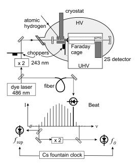
FIG. 1. Simplified experimental setup for comparison of the hydrogen 1S-2S transition frequency with a primary frequency standard (HV, high vacuum; UHV, ultrahigh vacuum). A modelocked femtosecond laser with repetition rate  $f_{\rm rep}$  emits the frequency comb which is broadened in a photonic crystal fiber.  $f_0$  is the carrier-envelope offset frequency.
