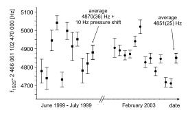
FIG. 2. Experimental results and averages for the 1999 and 2003 measurements of the absolute  $(1S, F = 1, m_F = \pm 1) \rightarrow (2S, F' = 1, m_F' = \pm 1)$  transition frequency in atomic hydrogen. The background pressure shift of +10 Hz as explained in [8] is added to the 1999 value.
