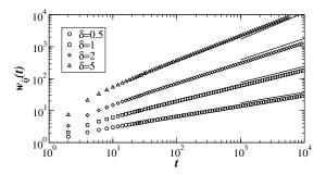
FIG. 4. Time evolution of  $w_{ij}$  during the growth of the network (m = 2 and  $N = 10^4$ ) for different values of  $\delta$ . The functional behavior is consistent with the predicted power laws  $t^b$ ,  $b = \delta/(1 + \delta)$ , shown by thick lines.
