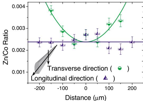
FIG. 1 (color online). Zn/Co ratio in a single crystal of CoPhOMe. The distribution of the dopant is reported for both longitudinal and transversal directions, scanned as shown in the drawing. Lines are guides to the eye.
