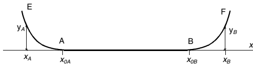
FIG. 3. Scheme for the quantification of curved GB portions close to the (100)_{\Sigma 3\text{CSL}} facet.
