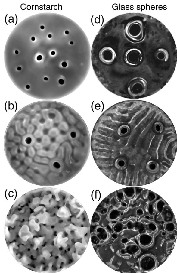
FIG. 1. Top view of a vibrated layer of an aqueous suspension of (a)–(c) cornstarch and of (d)–(f) glass microspheres (image diameter, 9.4 cm). White corresponds to the highest points, and black to depressions that reach near the container bottom. Holes without Faraday waves: (a)  $a = 12g$ ,  $f = 150$  Hz; (d)  $30g$ ,  $100$  Hz. Holes with Faraday waves: (b)  $12g$ ,  $60$  Hz; (e)  $27.3g$ ,  $92$  Hz. Delocalized state: (c)  $30g$ ,  $120$  Hz; (f)  $30g$ ,  $60$  Hz.
