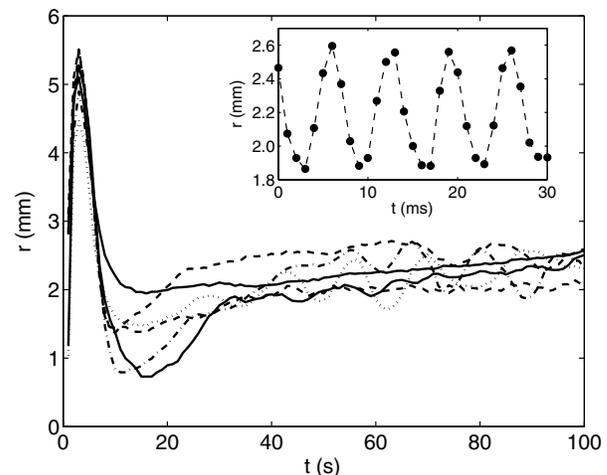
FIG. 3. Time evolution of the radii of six holes formed with a 2 s long puff of air. Holes grow during the forcing and then rapidly shrink after the air is cut off. Inset: hole diameter oscillates synchronously with the forcing; note time scale ( $a = 15g$ ,  $f = 150$  Hz).
