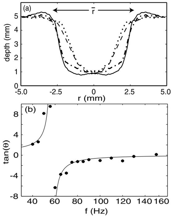
FIG. 4. (a) Vertical cross sections of holes at  $a = 14.5g$  (dashed and dotted lines) and  $a = 17g$  (solid and dot-dashed lines) for  $f = 150$  Hz. The two profiles for each acceleration show the extremes in a hole's shape, separated by one-half cycle. (b) The tangent of the phase lag versus frequency at  $a = 15g$ . The solid line is a fit to  $\alpha/[1 - (f/f_0)^2]$ , where  $\alpha$  and  $f_0$  are fitting parameters.
