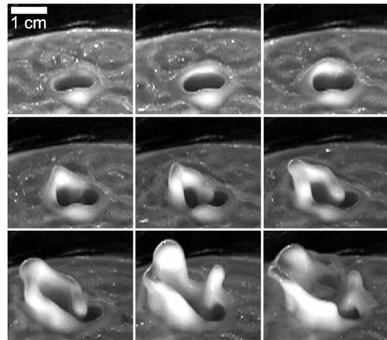
FIG. 5. Side view of the first steps toward the delocalized state in cornstarch. These photographs were taken every 0.9 s; time increases from left to right and top to bottom. An initial hump on the rim begins growing upward, reaches a maximum height, and then topples outward, enlarging the area of fluid motion. This process repeats until the entire surface of the liquid is active in the creation and destruction of vertical structures and voids [see Fig. 1(c)] ( $a = 25g$ ,  $f = 80$  Hz).
