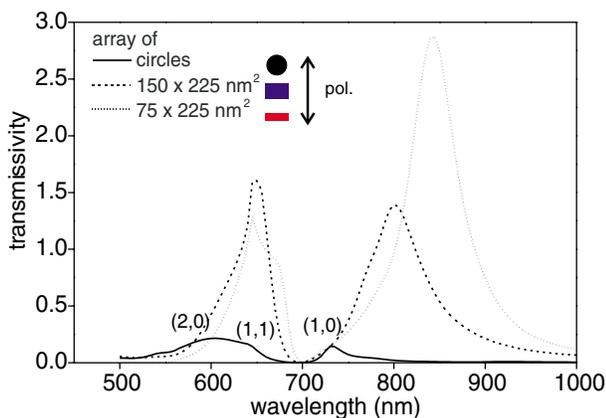
FIG. 3 (color online). Calculated transmissivity spectra for three different subwavelength hole arrays. The spectra are calculated for arrays consisting of circular holes (solid line),  $150 \times 225 \text{ nm}^2$  rectangles (dotted line), and  $75 \times 225 \text{ nm}^2$  rectangles (dashed line). The numbers between brackets specify the order of the maxima. The polarization of the incoming light was perpendicular to the long axis of the rectangles.
