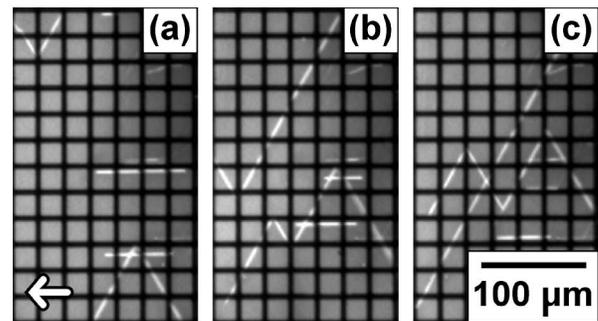
FIG. 3. Plan-view optical emission microscopy images showing the development of two rhombic stacking faults. The diode was biased between exposures at the current density of  $50 \text{ A/cm}^2$  for 1 min: (a) Two wedge-shaped Si(g) mobile fronts of the rhombic stacking faults are in the top left and bottom right regions. The  $8^\circ$  offcut toward the  $[11\bar{2}0]$  direction is marked with an arrow; (b),(c) the two bright wedges moved in opposite directions and passed each other.
