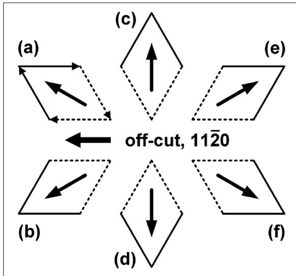
FIG. 2. Schematic analysis of Fig. 1. Each rhombus is a Shockley-type stacking fault bounded by a partial dislocation loop. The loops consist of solid and broken lines corresponding to luminescent, mobile and dark, stationary segments, respectively. The partial dislocation segments are all aligned along the Peierls valleys, the  $\langle 11\bar{2}0 \rangle$  directions. The arrow in each rhombus is the Burgers vector of the bounding partial dislocation loop.
