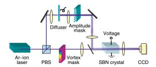
FIG. 3 (color online). Experimental setup. PBS: polarizing beam splitter; SBN: strontium barium niobate crystal.
