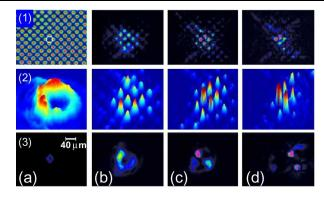
FIG. 4 (color online). Experimental observation of an optical vortex propagating with (rows 1,2) and without (row 3) an optically induced lattice. (a-1) the input pattern of the lattice, where the ring indicates the input vortex location; (a-2) and (a-3) the vortex beam at crystal output and input without bias field; (b)–(d) the vortex beam at output for bias fields of 600, 1200, and 3000 V/cm, respectively. Row 2: three-dimensional plots of vortex beam intensity.
