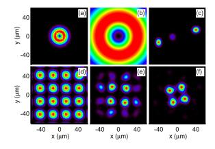
FIG. 1 (color online). Numerical results. (a) Input vortex and (d) linear lattice,  $I_0 = 10I_d$ . (b) Linear diffraction at z = 2 and (c) nonlinear propagation at z = 10 in a homogeneous medium. (e),(f) Discrete diffraction and discrete vortex soliton on the lattice, respectively, at z = 10 and  $V_0 = 16.09$ .
