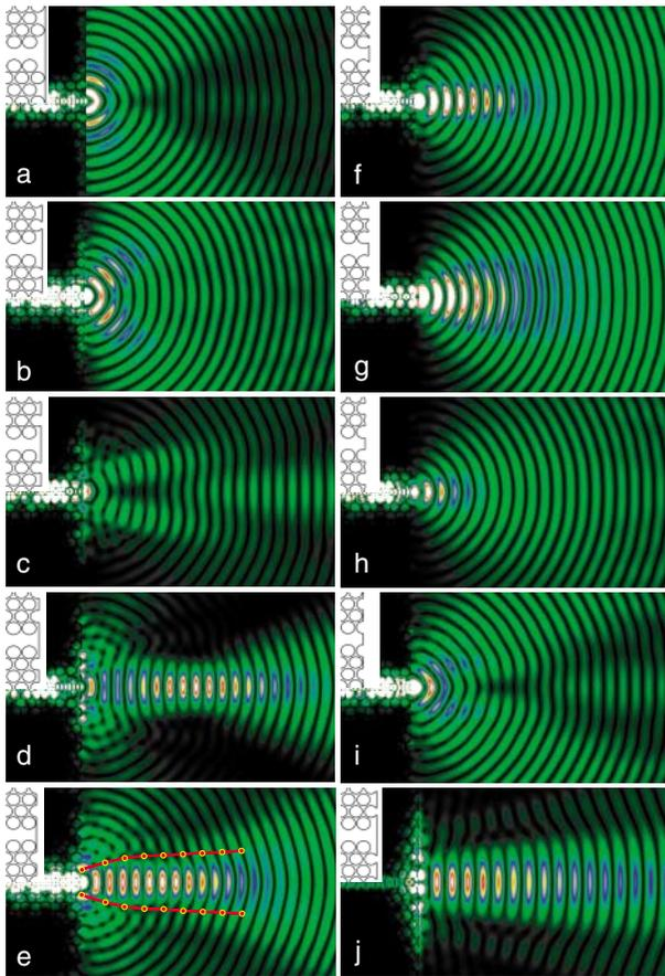
FIG. 3 (color). (a)–(i) Snapshots of the wave front and intensity distribution of light at  $\omega a/2\pi c = 0.39$ , exiting a photonic crystal waveguide for nine different structure terminations. The inset superposed on the upper left side of each graph displays the PC output termination. The symbols in (e) display the measured widths of the central spot at the corresponding locations. (j) The intensity distribution for the structure in (b) but at  $\omega a/2\pi c = 0.33$ .
