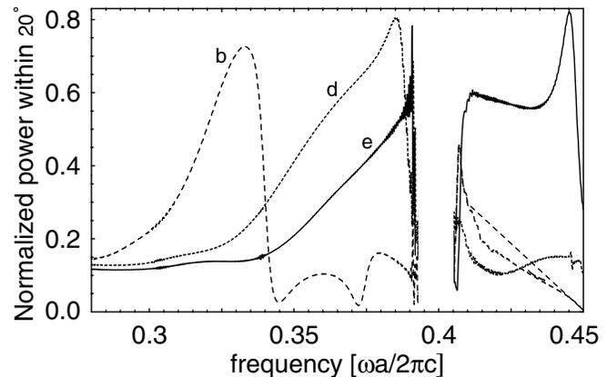
FIG. 4. Power transmitted within  $10^\circ$  of the waveguide axis as a function of  $\omega a/2\pi c$  for three different output terminations corresponding to those in Figs. 3(b), 3(d), and 3(e). The region around  $\omega a/2\pi c = 0.4$  corresponds to a mini stop band in the structure and is not suitable for guiding [16].
