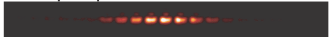
FIG. 4 (color online). Experimental results of a bright gap-soliton measurement, excited exactly at the top edge of band No. 2 (marked in Fig. 1), using a shaped input beam. Shown are photographs of the beam at the array output, for low and high powers. At low power, the input beam diffracts into about twice its initial width. At high power, a bright gap soliton is formed, traveling across the array at zero transverse velocity. We note that high index-step samples were used in this measurement, which possess a slightly double-humped modal shape of band No. 2, unlike the simulations shown in previous figures, where a smaller index step was assumed, which possess a single-humped modal shape of band No. 2.
