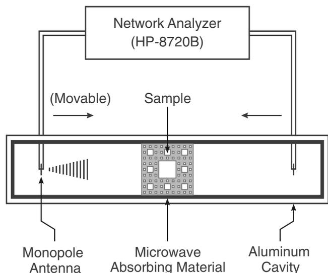
FIG. 2. Schematic illustration of experimental setup for the measurement of microwave transmission and reflection properties of a photonic fractal.
