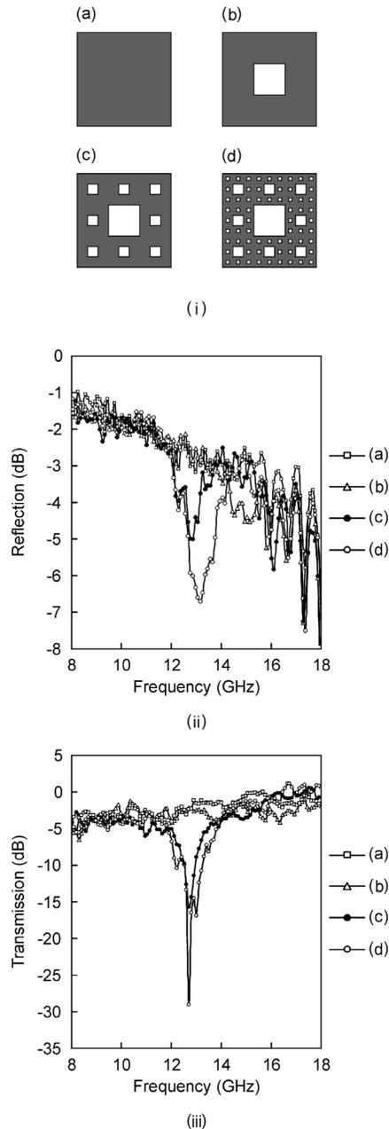
FIG. 3. (i) Illustration of the Menger sponges of stages 0, 1, 2, and 3. (ii) Reflection and (iii) transmission spectra of the Menger sponges of (a) stage 0, (b) stage 1, (c) stage 2, and (d) stage 3. A sharp attenuation maximum at around 12.8 GHz is observed in both the reflection and transmission spectra of the Menger sponge of stages 2 and 3. The  $Q$  factor of the 12.8 GHz mode is as large as 610 for the stage 3 sample.
