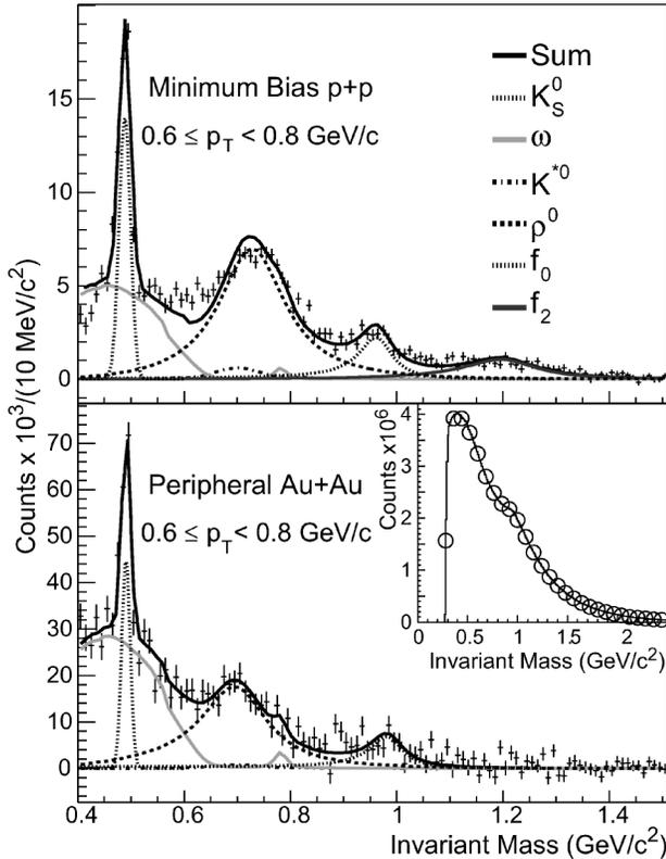
FIG. 1. The raw  $\pi^+\pi^-$  invariant mass distributions after subtraction of the like-sign reference distribution for minimum bias  $p+p$  (top) and peripheral Au+Au (bottom) interactions. The inset plot corresponds to the raw  $\pi^+\pi^-$  invariant mass (solid line) and the like-sign reference distributions (open circles) for peripheral Au+Au collisions.
