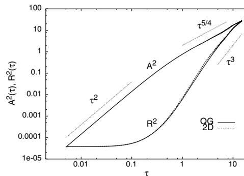
FIG. 4. Absolute dispersion,  $A^2$ , and relative dispersion,  $R^2$ , vs the time interval  $\tau = t - t_0$ , with  $t_0 = 5$ . Solid lines refer to QG and dashed lines to 2D. Dotted lines show the Richardson prediction for relative dispersion,  $R^2 \propto \tau^3$ , and the ballistic regime,  $A^2 \propto \tau$ , and the intermediate anomalous regime,  $A^2 \propto \tau^{5/4}$ , for absolute dispersion.
