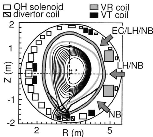
FIG. 1. Cross-sectional view of the JT-60U tokamak. VR (grey) and VT (black) coils are used to maintain equilibrium and control the plasma shape. The configuration shown in grey is used in the noninductive current ramp-up phase, while the black one is used in the advanced tokamak phase. The black one is a reconstructed equilibrium at  $t = 8.5$  s of the discharge shown in Fig. 2.
