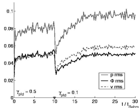
FIG. 2. Time evolution of the rms fluctuation amplitude of pressure (solid gray line), electrostatic potential (black line), and velocity (dashed line) for the case of a torus having  $\rho_* = 0.02$  and  $F_{\text{in}} = 0.2$ .
