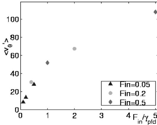
FIG. 7. rms ZF shearing rate as a function of the ratio of the injected heat flux to the collisionality, for the case of a torus with  $\rho_* = 0.02$ .
