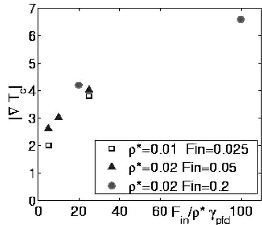
FIG. 8. Effective ion temperature gradient threshold as a function of the ratio of the injected flux to the collisionality, normalized to  $\rho_*$ .
