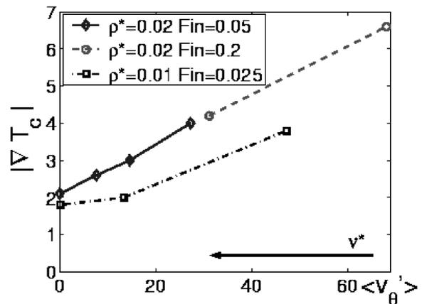
FIG. 6. Effective ion temperature gradient threshold as a function of the spatial rms ZF shearing rate, for the case of a torus with  $\rho_* = 0.02$  ( $\diamond$ ,  $\circ$ ) and  $\rho_* = 0.01$  ( $\square$ ).
