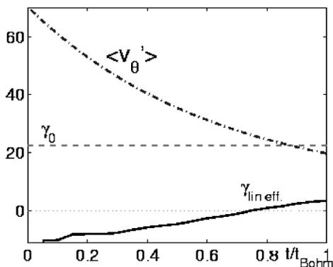
FIG. 4. Fluctuation energy growth rate (solid line) vs shearing rate (dash-dotted line); the linear growth rate  $\gamma_0$  is plotted (dashed line).
