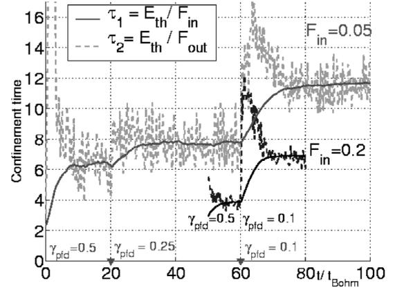
FIG. 1. Energy confinement times for a torus having  $\rho_* = 0.02$  and  $F_{\text{in}} = 0.05$  and  $0.2$ , evaluated as the ratio of the thermal energy to the injected flux,  $\tau_1$  (solid line), and the ratio of the thermal energy to the outgoing heat flux,  $\tau_2$  (dashed line).
