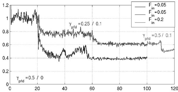
FIG. 3. Time evolution of the ratio between potential and pressure fluctuations for all the simulations with  $\rho_* = 0.02$ .
