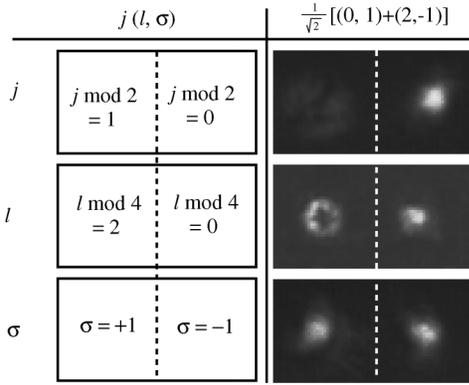
FIG. 5. Results for sorting superpositions of TAM states. The input mode was a superposition of  $l = 0, \sigma = +1$ , and  $l = 2, \sigma = -1$  so that  $j = +1$ .
