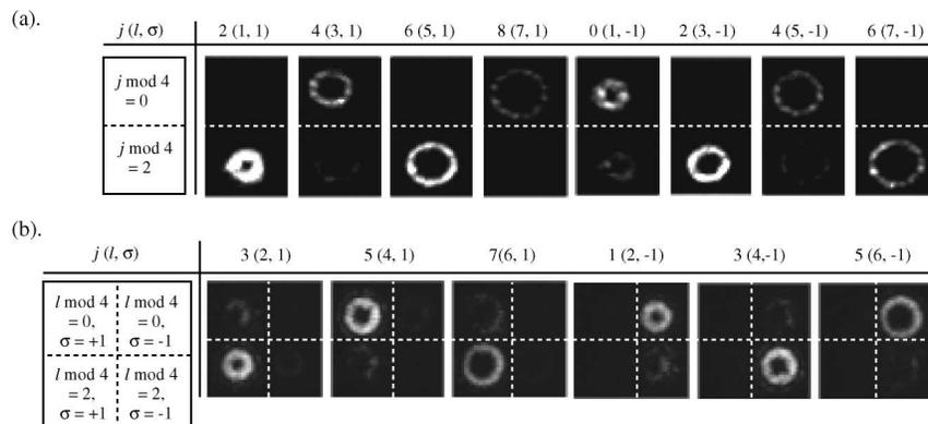
FIG. 4. Intensity outputs from various sorting schemes based on the total angular momentum. (a) Output from second stage sorting where the optical path of the photon is selected on the basis of the TAM. (b) Output from sorting first on the basis of the OAM state and then on the basis of the SAM state.
