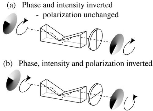
FIG. 3. The image and phase rotating prism acting in opposition with a conventional quarter-wave plate to leave the polarization state unchanged (a) or, in addition, to act as a half-wave plate (b).
