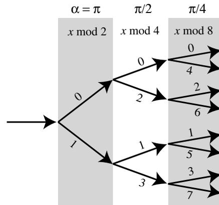
FIG. 2. The general sorting network for angular momentum. This cascade of interferometers can be used to sort photons on the basis of SAM, OAM, or TAM, where  $x$  represents  $\sigma$ ,  $l$ , or  $j$ , respectively.
