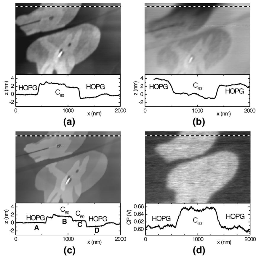
FIG. 1. NC-AFM measurement of  $C_{60}$  on HOPG. The topography is shown for  $V_{\text{bias}} = 0$  V (a) and  $V_{\text{bias}} = 1.34$  V (b). Topography (c) and simultaneously determined CP image (d) obtained by KPFM, with actively controlled  $V_{\text{bias}}$ . Corresponding line scans are shown below the images. All images are  $2 \times 1.35$   $\mu\text{m}$  measured at  $\Delta f = -10$  Hz.
