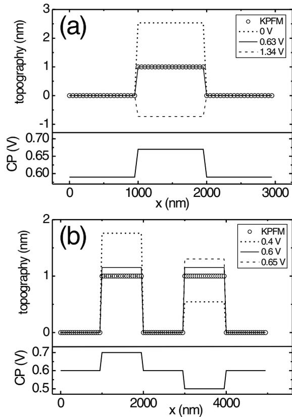
FIG. 3. The effect of electrostatic forces on the topography measurement in NC-AFM. (a) Simulation of two different materials (mimicking the experimental result of Fig. 1), where the CP is shown in the lower panel and the resulting topography for different  $V_{\text{bias}}$  in the upper panel. (b) Simulation of three different materials showing that for correct height measurements a KPFM method is mandatory. See text for details.
