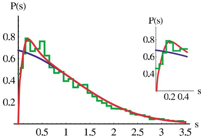
FIG. 4 (color). Comparison between the nearest neighbor spacing distribution in the deformed elliptical microresonator for  $kR \approx 75$  (green), best fit Berry-Robnik distribution (blue) and our analytical result (red); the inset shows the limit of small spacing in more detail.
