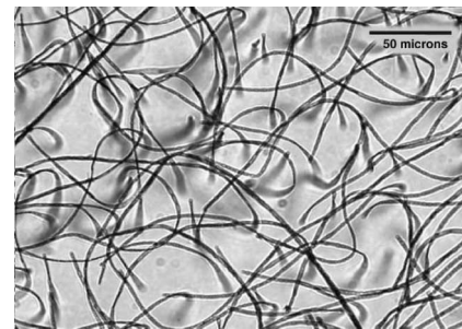
FIG. 1. Long flexible monodisperse filament, seen from above, made in a 200\ \mu\text{m} thick cell. The chains are bent by gravity after field removal.
