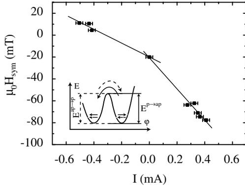
FIG. 4. External magnetic field  $H_{\text{sym}}(I)$  vs applied current  $I$  at which  $\langle \tau_{ap} \rangle = \langle \tau_p \rangle$ . Inset: schematic view of the potential profile, where  $\varphi$  represents the relative magnetization orientation of the Co layers. Straight lines are a guide for the eye.
