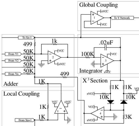
FIG. 3. Electronic circuit diagram of a unit oscillator of the overdamped Duffing oscillator arrays in Fig. 4. All circuit components and values are listed in the diagram. Op-amps are LM348N made by National Semiconductor.
