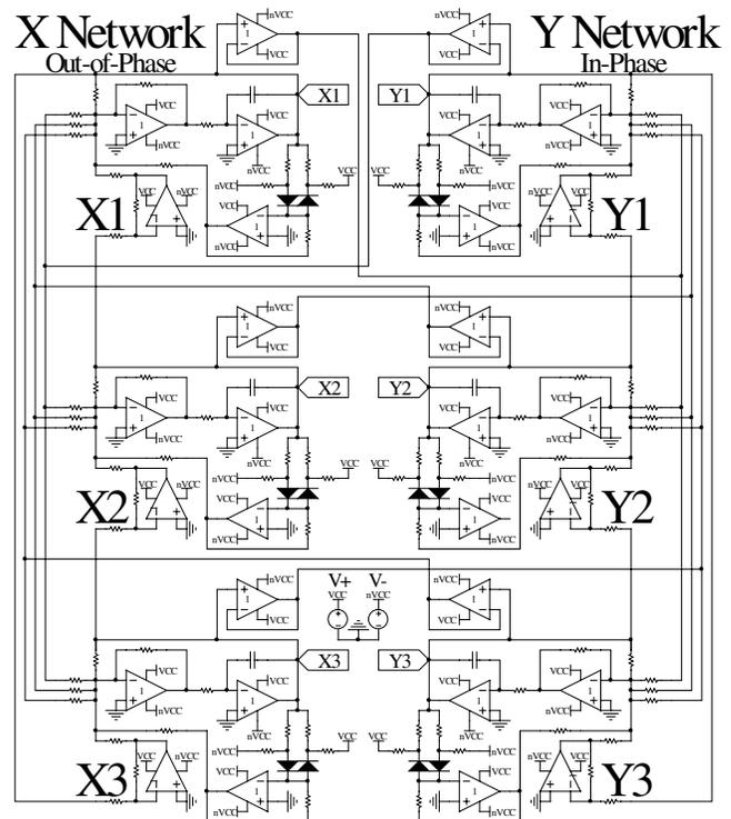
FIG. 4. Electronic analog of the network of two coupled arrays shown in Fig. 1. To guard against parasitic coupling between the arrays, each array is provided with its own power regulators.
