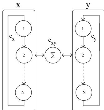
FIG. 1. Schematic diagram of a two-array network of coupled oscillators with  $N$  oscillators per array.
