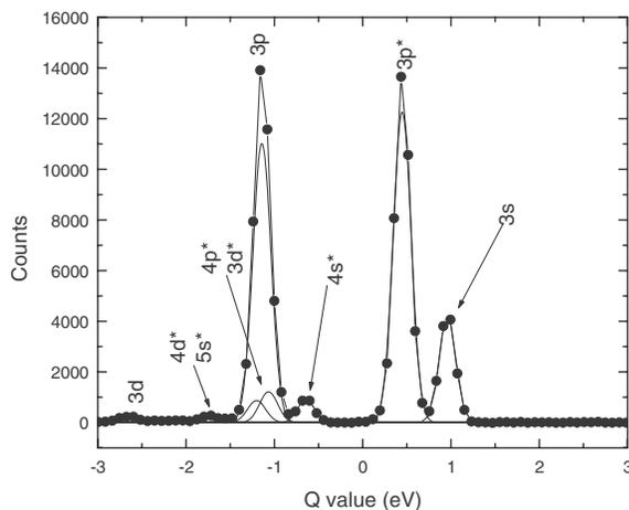
FIG. 1.  $Q$ -value plot for the  $7 \text{ keV Na}^+ + \text{Rb}$  collision system. Both lasers driving the  $5s\text{--}5p$  transition are on. Peak labels containing a star indicate channels where capture is from the  $5p$  state. Other peaks represent capture from the ground state. The solid line is the sum of Gaussian fits to the individual peaks.
