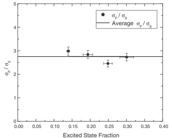
FIG. 3. Ratio of capture cross sections versus measured excited state fraction. Error bars are absolute.
