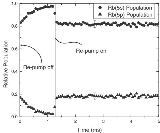
FIG. 4. Time dependence of relative Rb(5s) and Rb(5p) populations. At  $t = 0$ , the light from the “repump” laser was blocked. The vertical line near 1.2 ms indicates at which point the beam was turned back on. Representative error bars are absolute; relative error is smaller than the size of the points.
