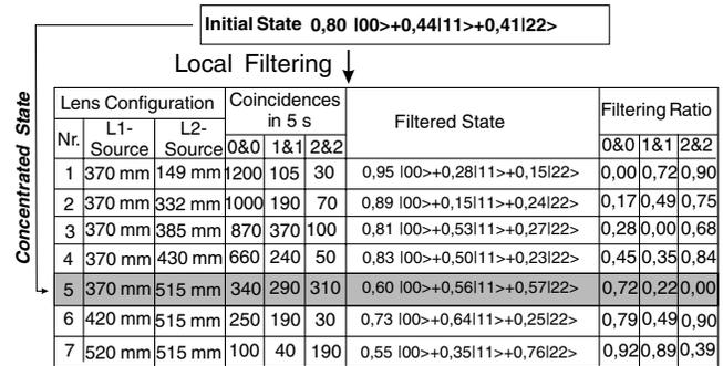
FIG. 3. “Procrustean” filtering method. Each lens configuration in the setup causes a specific filtering of the three modes  $LG_{00}$ ,  $LG_{0|1}$ , and  $LG_{0|2}$ . In general the filter density is different for each mode and depends on the positions of the two lenses L1 and L2. Specially the lens configuration 5 causes the concentration of the initial state. The concentrated state has nearly equal amplitudes. Typical errors for the amplitudes of the filtered states are about 0, 02.
