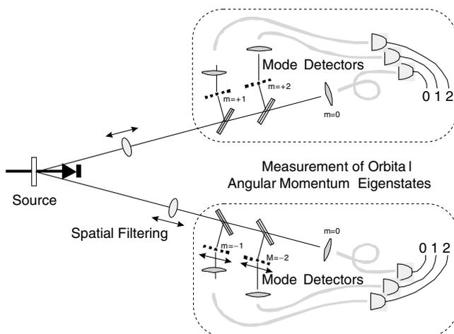
FIG. 1. Experimental setup for the entanglement concentration. After type-I spontaneous parametric down-conversion two lenses are used for spatial mode filtering by which the relative amplitudes between different LG modes are changed. The second part of the setup projects the photons onto the orbital angular momentum OAM eigenstates.
