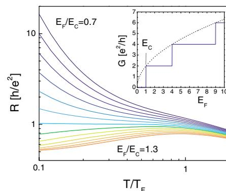
FIG. 2 (color online). Temperature dependence of the two-terminal resistance for various values of  $E_F$ . The inset shows the zero temperature dependence of the conductance as a function of  $E_F$  and the dotted line illustrates the overall square root dependence of the conductance steps.
