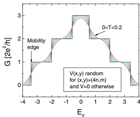
FIG. 1 (color online). Fermi energy dependence of the two-terminal conductance with  $V_{4n,m}$  random and all others zero. The results are obtained from the tight-binding Hamiltonian and for different temperatures.
