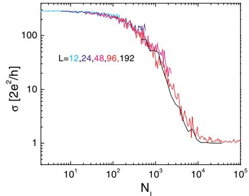
FIG. 4 (color online). The conductivity as a function of the number of impurities for different sizes and for  $-1 < V_2 < 1$ . Here only every second site is disordered.
