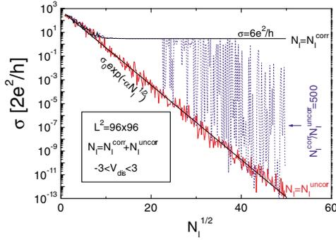
FIG. 5 (color online). The conductivity as a function of the number of impurities for different ratios of correlated to uncorrelated impurities. The straight line is the fit  $\sigma \sim \exp(-\alpha N_I^{1/2})$  and the dotted line corresponds to the intermediate case.
