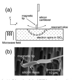
FIG. 1. (a) Schematic of the MRFM experiment. As the cantilever oscillates, the spins near the resonant slice are cyclically inverted, resulting in a small cantilever frequency shift. Cantilever position is detected using an optical fiber interferometer (not shown). (b) Scanning electron micrograph of the single-crystal silicon cantilever with the larger (micronsize) magnetic tip. The cantilever had a mass-loaded geometry in order to suppress motion of the tip for higher order flexural modes.
