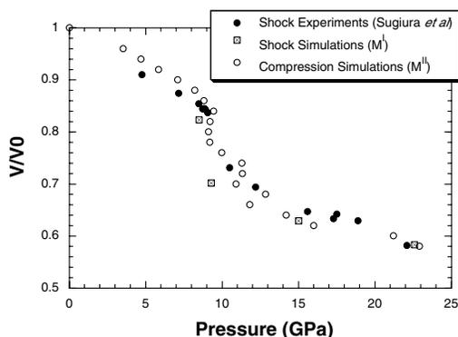
FIG. 1. Pressure-volume behavior calculated from MD simulations compared to experiments [4].
