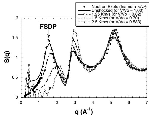
FIG. 2. Structure factor from  $M^{\text{I}}$  calculations. Experimental results for zero pressure are also included for comparison.
