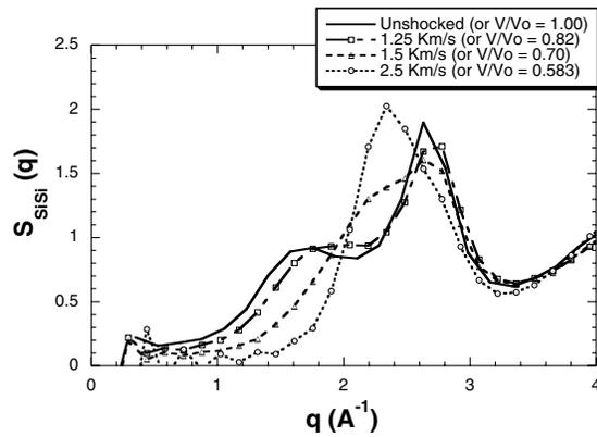
FIG. 3. Partial structure factor for Si-Si from shock simulations ( $M^I$ ).
