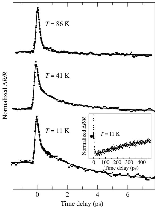
FIG. 1. Time resolved transient differential reflectivity  $\Delta R/R$  of an  $\text{MgB}_2$  thin film measured at three different temperatures. Both the pump and probe wavelengths were 800 nm and the average pump power was 1 mW. The inset shows the  $\Delta R/R$  response below  $T_c$  in a much longer time window.
