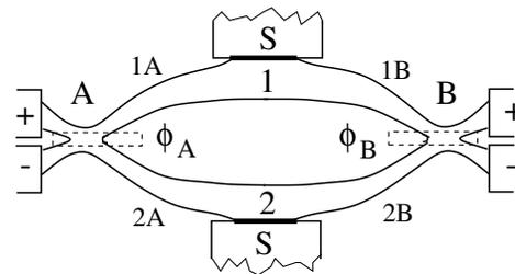
FIG. 1. The system. A single superconductor (S) is connected to four normal arms via two tunnel barriers (1 and 2) (thick black lines). The arms are joined pairwise in beam splitters A and B and end in normal reservoirs + and -.
