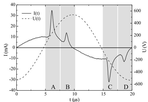
FIG. 4. Oscillogram of the discharge current  $I$  (solid line) and the supply voltage  $U$  (dashed line) corresponding to the concentric-ring pattern shown in Fig. 5.
