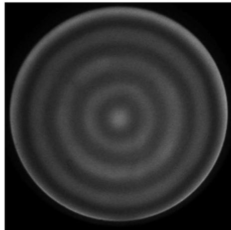
FIG. 1. Sample of the concentric-ring pattern observed in barrier gas discharge in nitrogen. Peak to peak value of supply voltage  $U_{pp} = 1050$  V; gas pressure  $p = 2.5$  hPa. The image was made by means of a video CCD camera with exposure time of 40 ms. Diameter of the gas-discharge area  $D = 40$  mm.
