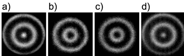
FIG. 5. Sequence of single discharge pulses of the concentric-ring pattern observed in the barrier gas discharge in nitrogen. Peak to peak value of the supply voltage  $U_{pp} = 1050\ \text{V}$ , shown in Fig. 4; gas pressure  $p = 2.5\ \text{hPa}$ . Images (a)–(d) represent patterns corresponding to the stripes A–D in Fig. 4, respectively. Each image is a sum over 50 frames made with the DiCAM-2 camera with exposure time of  $2.5\ \mu\text{s}$ .
