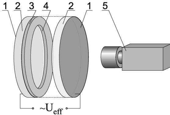
FIG. 2. Schematic representation of the discharge cell. The cell contains transparent ITO electrodes (1), deposited on glass plates (2), and spacer (3), which, together with glass plates (2), form the discharge area (4). Discharge is observed with a camera (5). The spacer contacts both glass plates. The front glass plate is shifted on the scheme to the right in order to show the discharge area.
