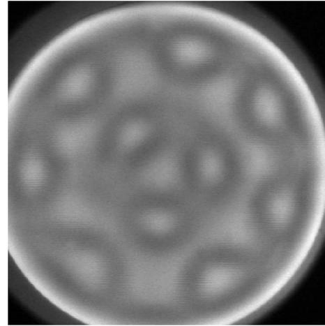
FIG. 3. Sample of the destabilized concentric-ring pattern observed in the barrier gas discharge in nitrogen. The peak to peak value of the supply voltage  $U_{pp} = 1050$  V; discharge pressure  $p = 4.0$  hPa. The image was made by means of a video CCD camera with exposure time of 40 ms.
