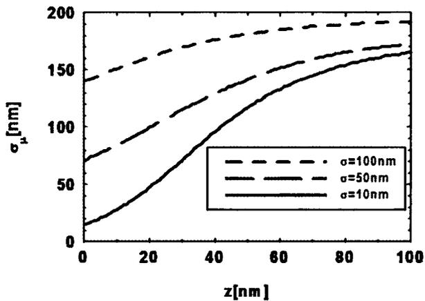
FIG. 1. Field coherence length  $\sigma_\mu$  as a function of distance  $z$  from the surface and calculated for different values of the source correlation length  $\sigma$  as indicated. The calculations account for both homogeneous and inhomogeneous contributions.
