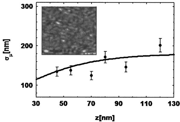
FIG. 3. Measured near-field coherence length as a function of the distance  $z$  from the surface. The inset shows a typical near-field intensity distribution.
