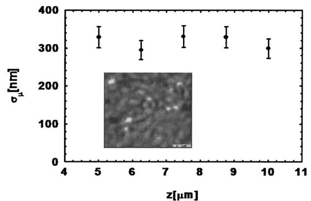
FIG. 2. Measured far-field coherence length as a function of the distance  $z$  from the surface. The inset shows a typical far-field intensity distribution.
