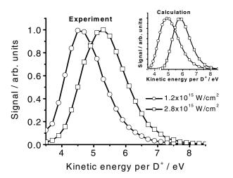
FIG. 3. Deuteron kinetic energy spectra for a 10.5 fs duration, circularly polarized pulse with an intensity of  $1.2 \times 10^{15} \ \text{W/cm}^2$  (circles) and  $2.8 \times 10^{15} \ \text{W/cm}^2$  (squares). Inset: calculated spectra corresponding to  $1.2 \times 10^{15} \ \text{W/cm}^2$  (dashed line) and  $2.8 \times 10^{15} \ \text{W/cm}^2$  (solid line).
