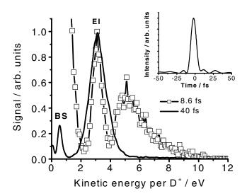
FIG. 1. Deuteron kinetic energy spectra at an intensity of  $5 \times 10^{14} \text{ W/cm}^2$  for linearly polarized pulse at durations of 40 fs (solid line) and 8.6 fs (squares). The time-dependent intensity profile of the 8.6 fs pulse is shown in the inset. BS: bond softening; EI: enhanced ionization.
