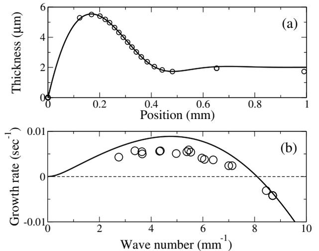
FIG. 2. Experimental measurements (circles) are compared with theoretical predictions (lines) of the slip model for the spreading of thin liquid film on a solid substrate. Error bars on the experimental data are less than the symbol size. (a) The capillary ridge behind the contact line (located at the origin) is the dominant topographical feature of the streamwise profile of an unstable spreading film. (b) The dispersion relation for a spreading film with a profile shown in (a).
