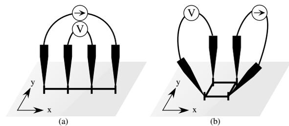
FIG. 1. Schematic drawings of the four-point probe method in (a) linear and (b) square arrangements. The probes are equidistant from each other. Current and voltage probes are shown.
