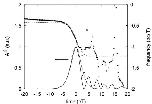
FIG. 2. A FEL pulse calculated for the 800th round trip. Intensity profile (solid line) and instantaneous frequency detuning normalized by the carrier period (+) are plotted for a temporal variable as optical cycles of carrier frequency. Dotted lines are results from chirped-sech<sup>2</sup> fitting,  $\alpha = 1.1$  and  $\tau_d/T = 2.7$ .
