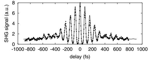
FIG. 4. A fringe-resolved SHG signal from the JAERI-FEL (dots). The solid line is a fitted curve by the chirped-sech<sup>2</sup> pulse,  $\alpha = 1.47$  and  $\tau_d/T = 2.32$ .
