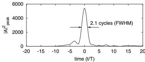
FIG. 3. Intensity profile of a FEL pulse after numerical chirp compensation applied to the pulse in Fig. 2.
