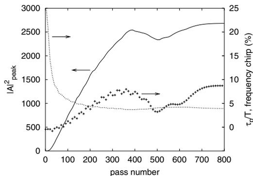
FIG. 1. Numerically calculated FEL pulse evolution for the JAERI-FEL parameters. Peak intensity (solid line), FWHM duration as optical cycles (dotted line), and a frequency chirp inside FWHM duration (+).
