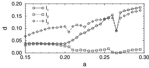
FIG. 3. Critical coupling curves.  $l_1$  corresponds to the onset of CPS, i.e., below this line the oscillations are not synchronized, and above this line the phase and frequency locking conditions are fulfilled;  $l_2$  corresponds to the transition of one of the zero LEs negative values; and  $l_3$  corresponds to zero crossing of one of the positive LEs. Note that in this figure we do not separate the cases where the synchronization occurs between regular and chaotic oscillations.
