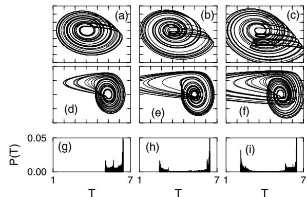
FIG. 1. Upper panel (a)–(c): projections of the attractors of the Rössler systems (1) onto the plane  $(x, y)$ ; middle panel (d)–(f): projections onto  $(\dot{x}, y)$ ; lower panel (g)–(i): distribution of the return times  $T$ . The parameters are  $\omega = 0.98$  and  $a = 0.16$  (a),(d),(g),  $a = 0.22$  (b),(e),(h), and  $a = 0.28$  (c),(f),(i).
