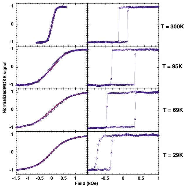
FIG. 1 (color online). Hysteresis loops with the field applied perpendicular (hard axis) and parallel (easy axis) to the FeF<sub>2</sub>  $c$  axis at various temperatures. The lines for the hard-axis data are fits using a coherent rotation model and the energy expression from Eq. (1), while the lines for the easy axis data are just guides to the eye.
