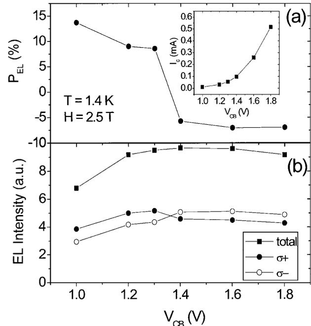
FIG. 4. The collector/base bias dependence of  $P_{\text{EL}}$  (a) and EL intensities (b) at 2.5 T. The inset in (a) shows the hole current as a function of  $V_{\text{CB}}$ . The emitter/base bias is  $V_{\text{EB}} = -2.06$  V.
