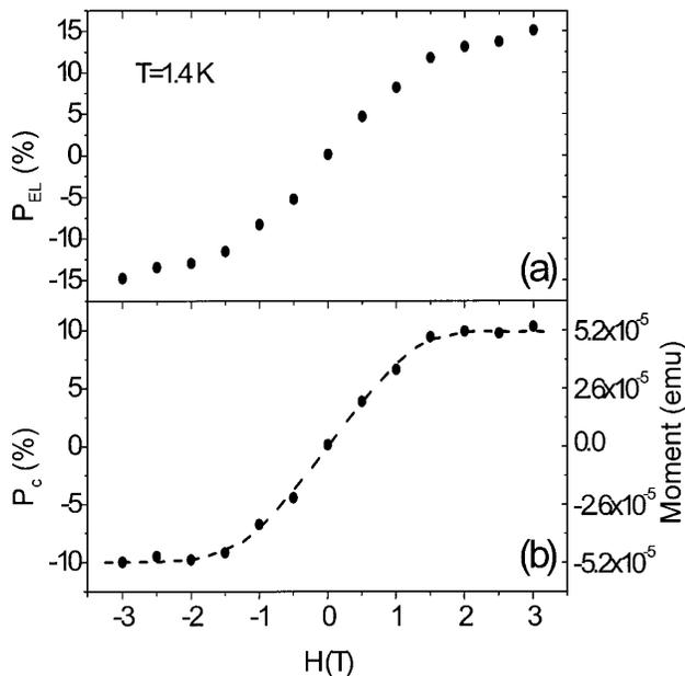
FIG. 3. The measured EL polarization  $P_{\text{EL}}$  (a) and the polarization after subtracting a linear background  $P_C$  (b) as a function of magnetic field at 1.4 K. The bias conditions are the same as those in Fig. 2. The dashed line in (b) shows the magnetic moments of the FM layers measured with a SQUID magnetometer at 10 K.
