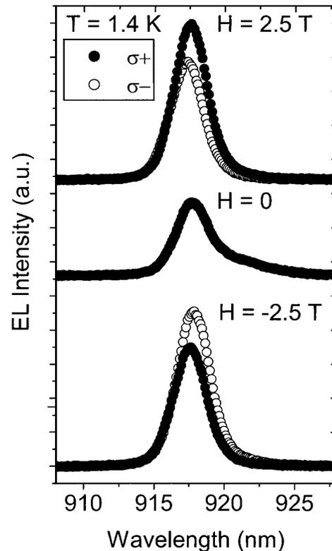
FIG. 2. Wavelength dependence of electroluminescence measured in magnetic fields of 2.5 T, 0, and  $-2.5$  T at 1.4 K. The solid and open circles represent  $\sigma^+$  and  $\sigma^-$  polarization components, respectively. The bias conditions are  $V_{\text{EB}} = -2.06$  V,  $V_{\text{CB}} = 1.0$  V.
