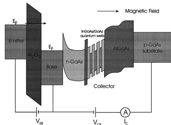
FIG. 1. Schematic energy band diagram of a magnetic tunnel transistor merged with a quantum well light-emitting diode collector. The emitter/base bias  $V_{EB}$  controls the energy of the injected hot electrons. The collector/base bias  $V_{CB}$  can be used to adjust the band bending of the LED.
