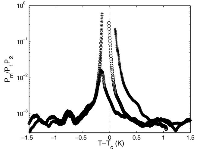
FIG. 4. Temperature dependence of the normalized amplitude  $P_m/P_1P_2$  (arbitrary units) for three different densities:  $\rho \approx 0.97\rho_c$  (\*),  $\rho \approx 0.95\rho_c$  (O),  $\rho \approx 0.905\rho_c$  ( $\diamond$ ).
