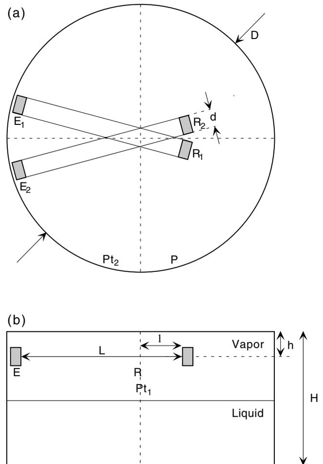
FIG. 1. Sketch of the experimental setup. (a) Top view, (b) side view.  $E_i$ : sound emitters,  $R_i$ : sound receivers,  $P_{t_i}$ : platinum resistors,  $P$ : pressure transducer.  $D = 200$  mm,  $L = 107$  mm,  $l = 30$  mm,  $H = 100$  mm, and  $h = 25$  mm.
