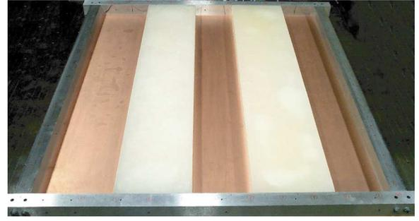
FIG. 2 (color online). Photograph of the cavity with top and antennas removed. The sidewalls have height  $H = 4.341(3)$  cm. The two paraffin wax bars fill the length  $L$  and height  $H$ .
