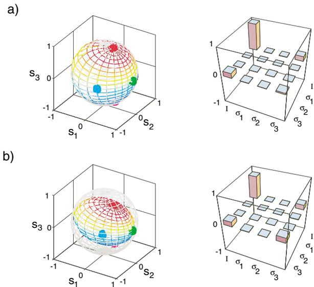
FIG. 4 (color). Geometric mappings and  $\chi$  matrices for (a) coherent and (b) incoherent partially polarizing processes. The former was implemented using two glass microscope slides near Brewster’s angle [ $T_H \sim 88\%$ ,  $T_V \sim 45\%$ ]. The latter was simulated by inserting a horizontal polarizer 50% of the time. (Real components shown; imaginary contributions  $<1\%$ .)
