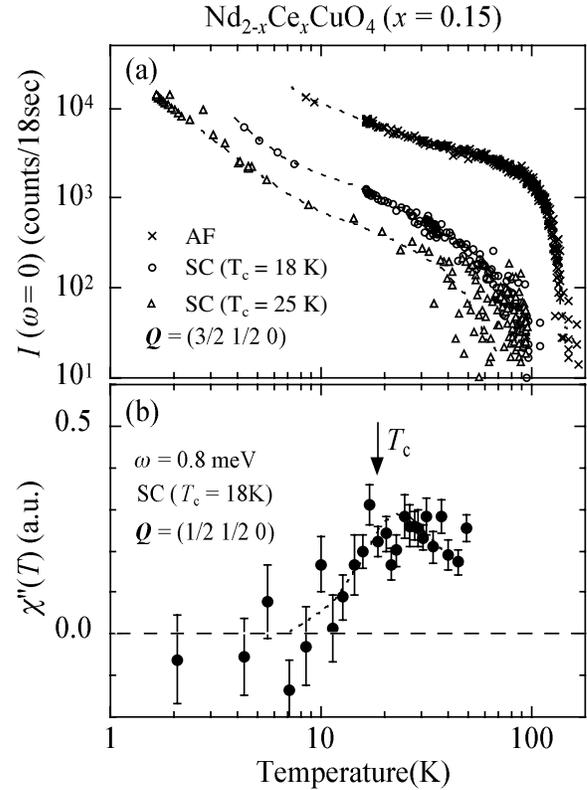
FIG. 1. (a)  $T$  dependence of the elastic magnetic peak intensities of NCCO ( $x = 0.15$ ) at  $(3/2 \ 1/2 \ 0)$  measured from an as-grown insulating (crosses) and the two reduced SC single crystals with  $T_c = 18$  K (open circles) and 25 K (open triangles). (b)  $T$  dependence of dynamical susceptibility  $\chi''(\omega = 0.8 \text{ meV})$  at  $(1/2 \ 1/2 \ 0)$  obtained from the reduced sample of NCCO ( $x = 0.15$ ,  $T_c = 18$  K). Dotted curves are to guide the eye.
