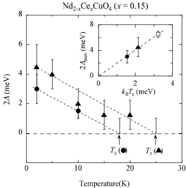
FIG. 4.  $T$  dependence of the spin gap,  $2\Delta$  for the  $n$ -type SC cuprate NCCO ( $x = 0.15$ ) with  $T_c = 18$  K (filled circles) and 25 K (filled triangles). Dotted lines are guides to the eye. At  $T_c$ , the spin gap is absent for both NCCO samples. The inset shows  $2\Delta_{\text{max}}$  versus  $k_B T_c$  obtained from our samples and LSCO ( $x = 0.15$ ) (open square, data taken from Ref. [12]).
