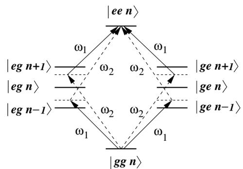
FIG. 2. Excitation scheme of pair of ions with ground state  $|g\rangle$  and excited state  $|e\rangle$  by bichromatic laser fields of equal and opposite detuning  $\delta$ .  $n$  denotes the quantum number of trap oscillation.
