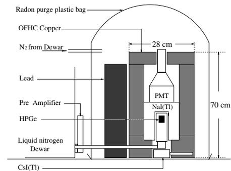
FIG. 1. Schematic layout of the HPGe with its anti-Compton detectors as well as inner shielding and radon purge system.
