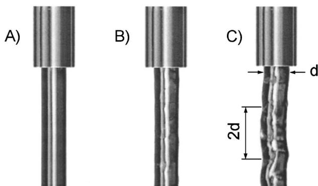
FIG. 1. Direct observation of the extrusion for different speeds for a 0.4% borax solution: (a) for the lowest speed ( $Wi = 2.8$ ) the surface is smooth (b) intermediate speed ( $Wi = 4.9$ ): development of a small roughness (c) at the highest speed ( $Wi = 8.4$ ) the melt fracture is well developed.
