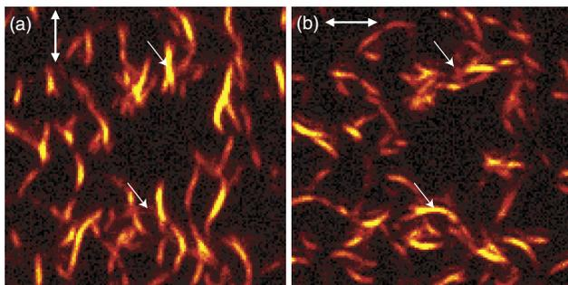
FIG. 1 (color online). Confocal Raman images of SWNT bundles produced by arc discharge on glass acquired by detecting the intensity of the *G'* band ( $\nu = 2615 \text{ cm}^{-1}$ ) while raster scanning the sample (without metal tip, scan area  $15 \times 15 \mu\text{m}$ ) for vertical (a) and horizontal polarization (b) of the laser excitation at 633 nm. The arrows indicate tubes which are oriented completely perpendicular to one polarization direction demonstrating the polarization contrast.
