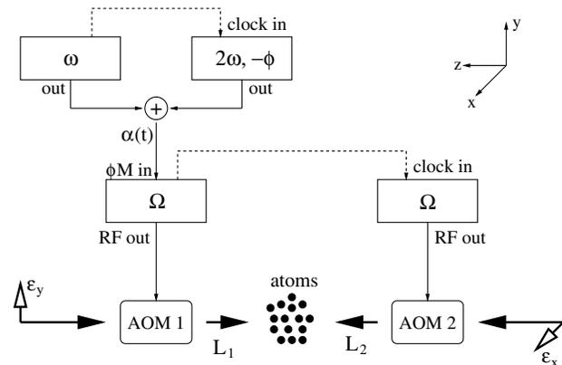
FIG. 1. Sketch of the experimental setup. The phase of the laser field  $L_1$  is  $-kz - \omega_L t + \alpha(t)$ , while the phase of the field  $L_2$  is  $kz - \omega_L t$ . Here  $\omega_L$  includes the frequency shift  $\Omega$  produced by the acousto-optic modulators.
