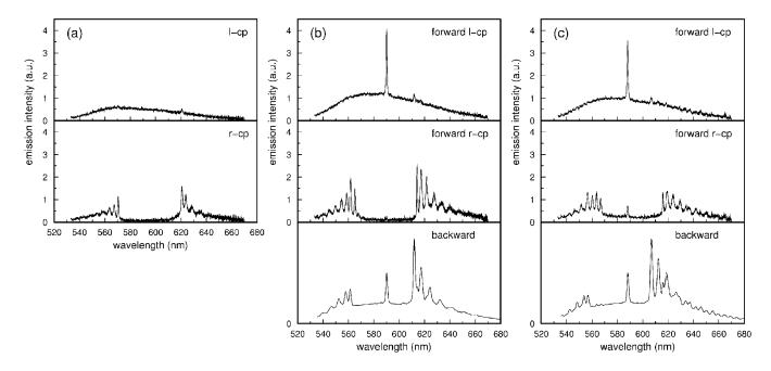
FIG. 3. Fluorescence of cholesteric films. (a) Single layer: l-cp (top) and r-cp (bottom) emission contributions. (b), (c) Fluorescence at two spots of the double layer with small (b) and large (c) mismatch of the cholesteric pitch: l-cp (top) and r-cp (middle) forward emission contributions, and total backward emission (bottom, not corrected for the polarization dependent detection sensitivity).
