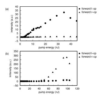
FIG. 5. Laser emission of the defect mode (a) and the band edge mode (b) as a function of pump energy.
