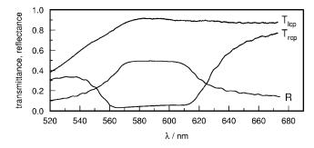
FIG. 6. Reflectance (*R*) and circularly polarized transmittances  $(T_{1-cp}, T_{r-cp})$  of the double layer system.
